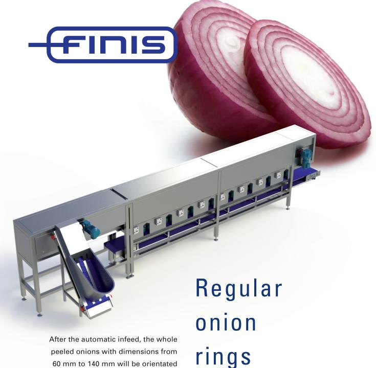
After the automatic infeed, the whole peeled onions with dimensions from 60 mm to 140 mm will be orientated automatically by a vibrating system. In the second stage the onions will be cut in regular slices by means of rotating knifes. The thickness of the rings is easy to adjust to different sizes. This machine works excellent in combination with our FUAS onion peeling line, but is also suitable to operate as a standalone ring slicer. The FRGR will process 3.600 to 7.200 onions per hour.
